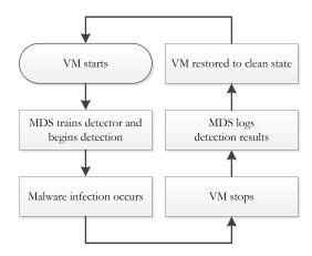
Fig. 5. Flow chart of malware testbed execution
