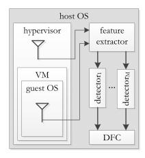
Fig. 2. Malware detection system architecture
